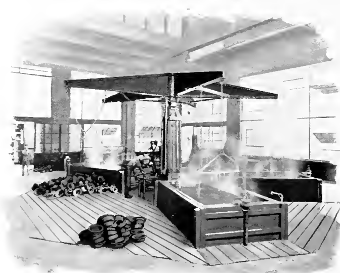
Mesta Pickling Machine Pickling Stamped Metal Parts
